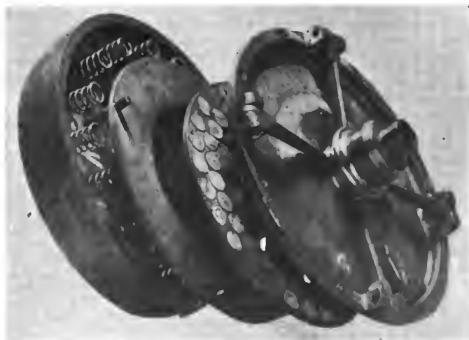
Knox Three-Plate Clutch Disassembled, Showing Cork Inserts
